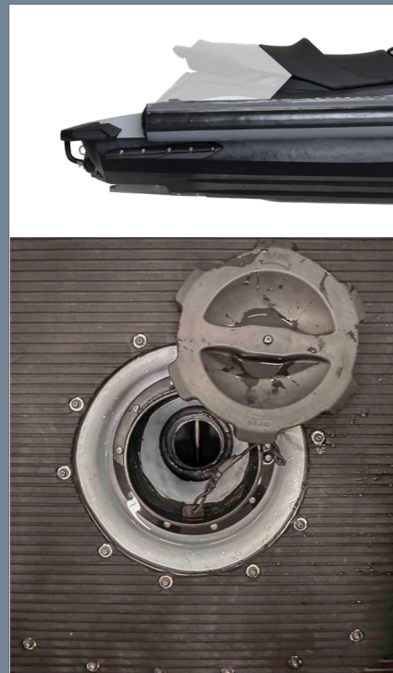
Aft deck - Single seater - Cleaning hatch for Water Jet intake - Load area
